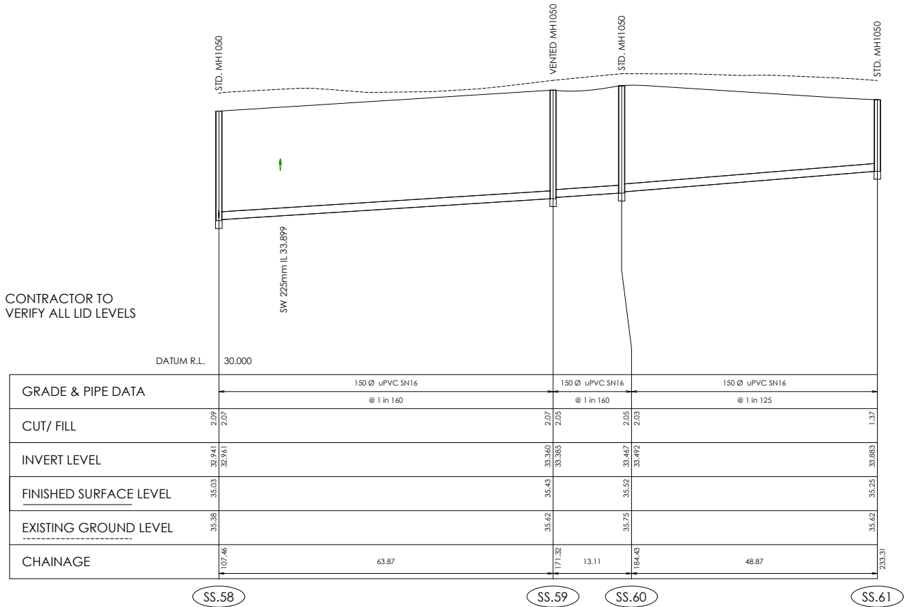
SEWER LONGSECTION SS.58 TO SS.61
