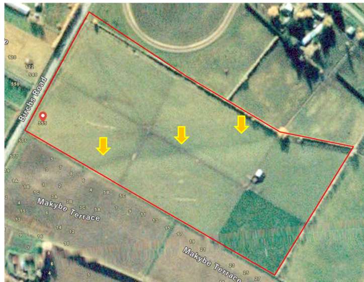
Figure 3: Photo sourced from Canterbury Maps showing apparent drainage feature (arrows),
