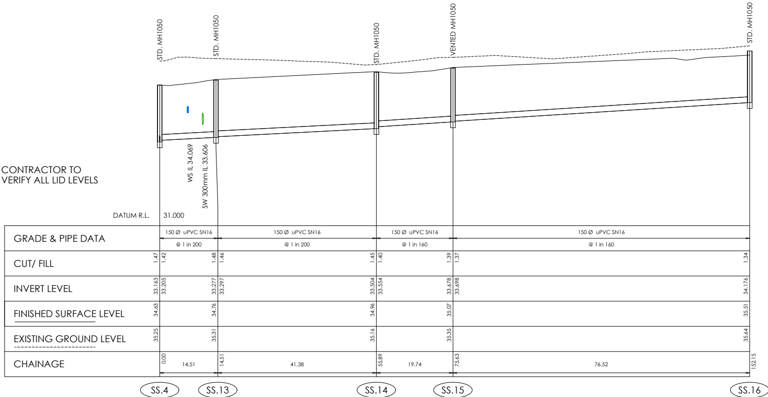
SEWER LONGSECTION SS.4 TO SS.16
