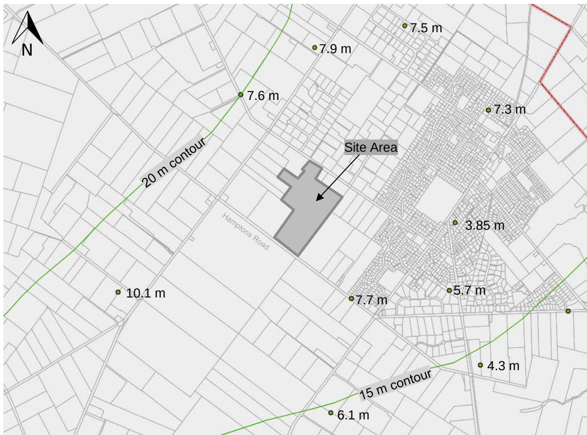
Figure 4: ECan Regional Piezometric Elevation Contours and Piezometric Wells used in various published groundwater studies.
